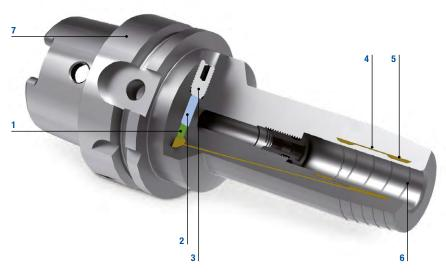
When clamping using hydraulic clamping technology, even pressure is built up in a sealed chamber system using a clamping screw and a piston. This pressure is transmitted to the tool via the built-in expanding sleeve.
