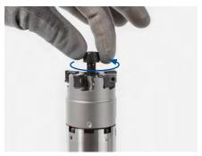
Unscrew the milling cutter clamping screw from the threaded bore and remove it.
