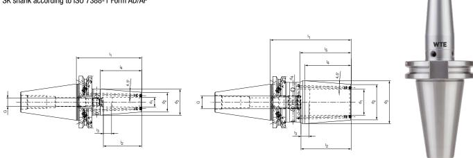
Design with two cooling channel outlets, resealable I Preferred series available from stock
