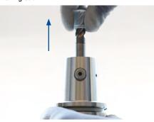
1. Remove the tool from the mill chuck's location bore.
