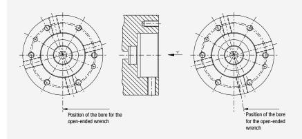
Spindle connection contour for adapter flange for short spindles in accordance with MN5000-13
