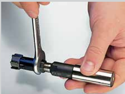
Tighten the adjusting nut by hand in the direction of the arrow.
