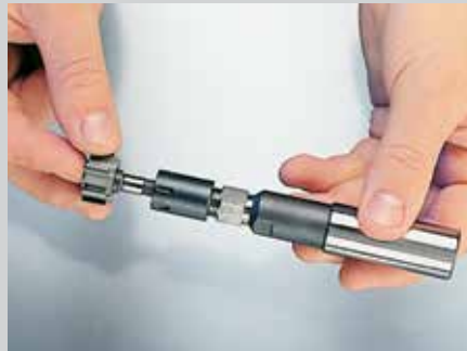
Screw in taper screw with cutting ring as far as the stop on the holder.
