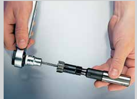
Tighten taper screw with torque key as shown in the guideline table.
