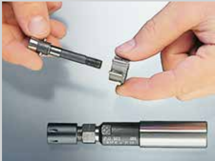
Slide cutting ring onto taper screw (cutting edges at front).
