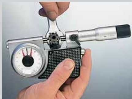
Set the cutting ring by tightening the adjusting nut to the nominal dimension. Measuring blades are marked behind the blade by a mark, a number or a boss.
