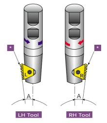
\* Important! Tool offset length and diameter for conical inserts should be measured on the first tooth.
