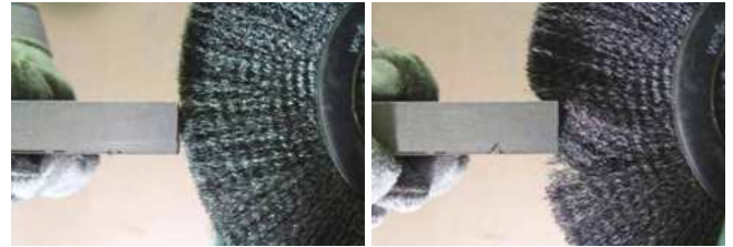
Correct Wire Tips Doing the Work
