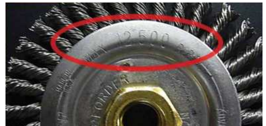
Match the RPM rating of the power brush to the tool being used. The RPM of the tool should never exceed the RPM of the power brush.
